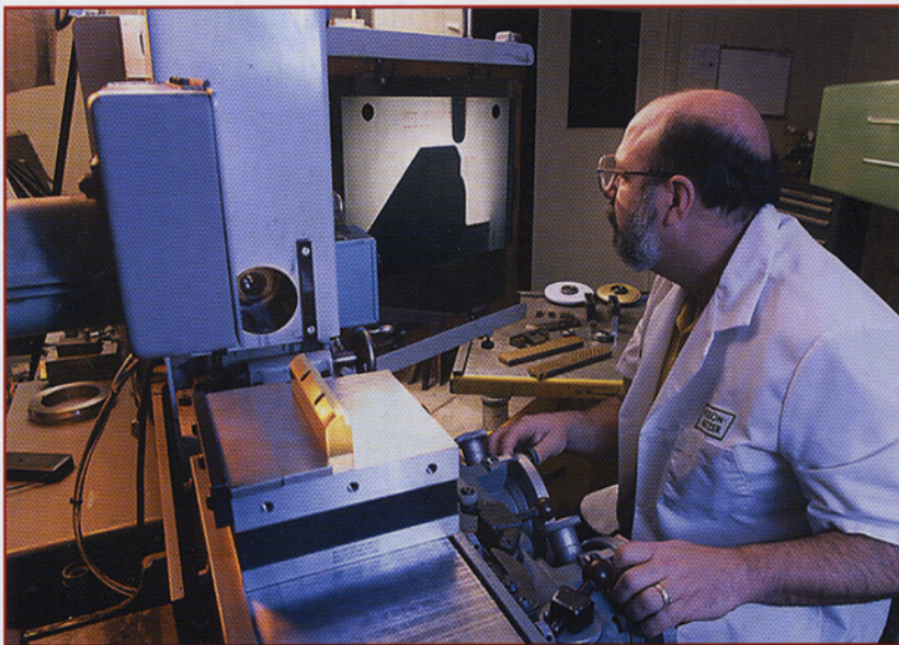
A machinist performs visual grinding of tooling components at Durham, CT-based Hobson and Motzer. Photo courtesy of Hobson and Motzer.
